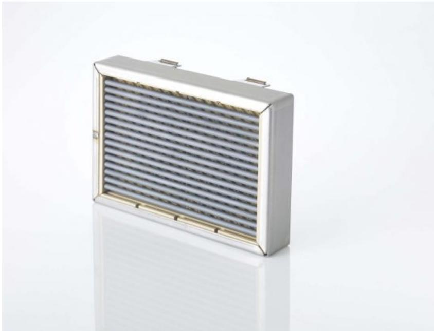
In the market since more than 10 years, our E emitters, GemE (for Ircon-Solaronics systems, 143 x 200mm) and GerE (for competitor systems, 150 x 200mm), benefit from two high-technology screens for higher infrared efficiency and a solid ceramic material known for its excellent mechanical properties and offer around 10% higher direct efficiency. The emitters are optimised thanks to a specific surface treatment to efficiently operate at high temperatures. Input power: from 4 to 12 kW.
